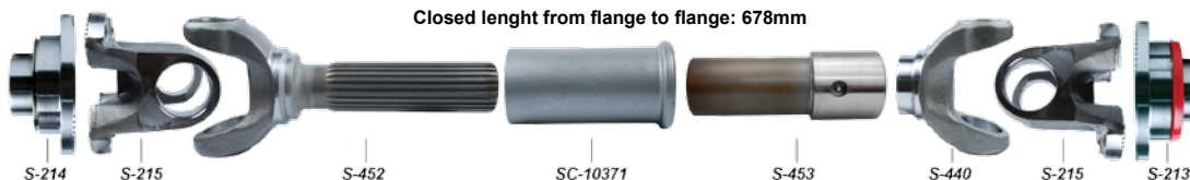
Closed length from flange to flange: 678mm
